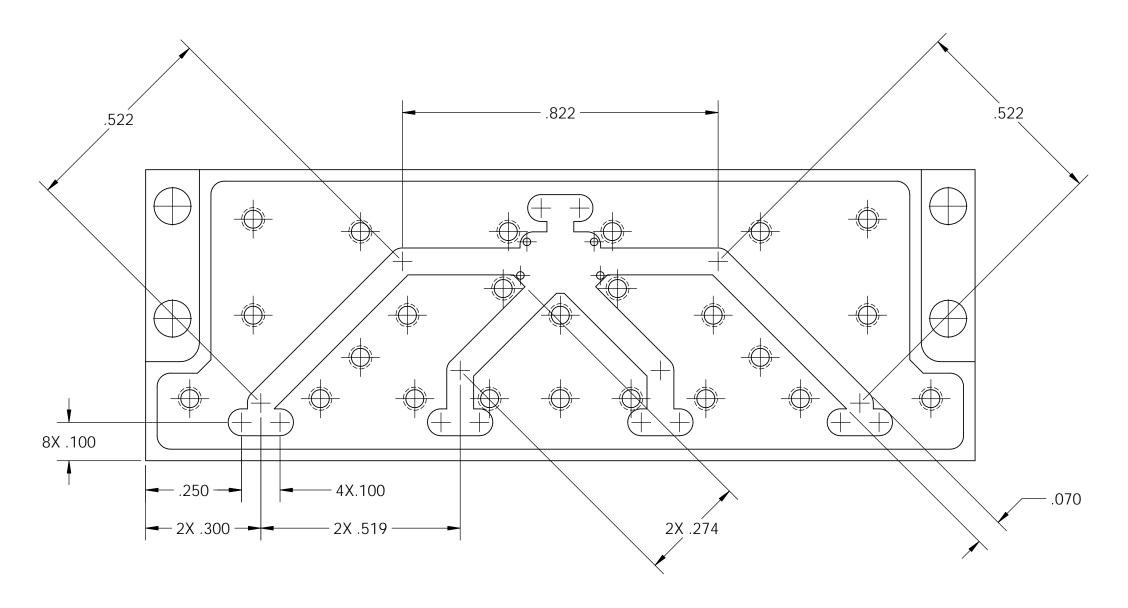
Aligned dimensions are placed so the horizontal dimensions can be read from the bottom of the drawing sheet and the vertical can be read from the right side of the drawing sheet.
