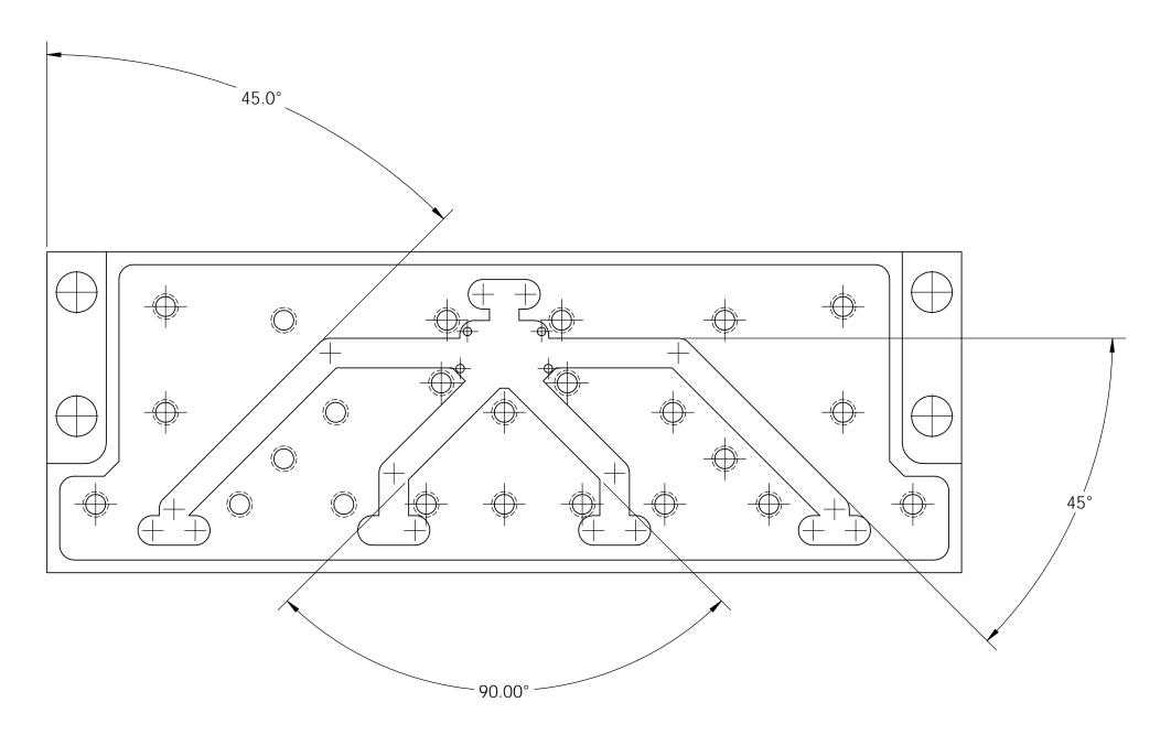
Aligned dimensions are placed so the horizontal dimensions can be read from the bottom of the drawing sheet and the vertical can be read from the right side of the drawing sheet.
