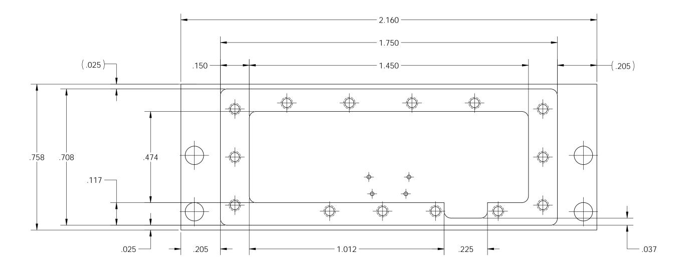
Reference dimensions on drawing are enclosed within parentheses.
