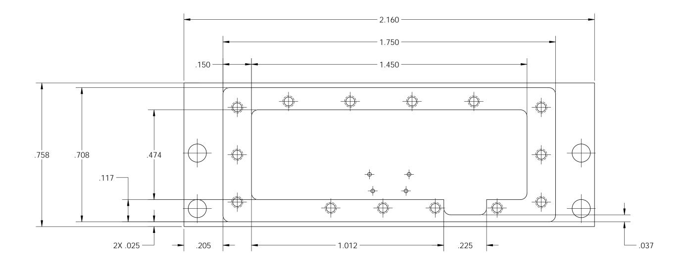
Unidirectional dimensions are placed so they can be read from the bottom of the drawing sheet. This method is commonly used in mechanical drawing.
